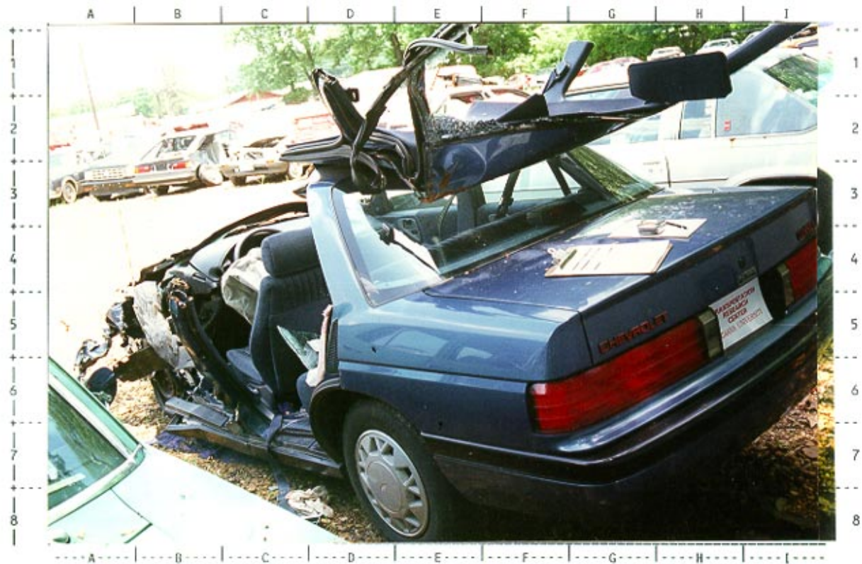
# 42 -- Left back (45 degree angle) view of '91 Chevrolet Corsica; NOTE: direct contact to left A-pillar and roof corner (cells D1--E3)
